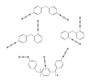
**Figure-1.** Illustrative structures of methylenediphenyl diisocyanate (MDI) and polymeric methylenediphenyl diisocyanate PMDI
